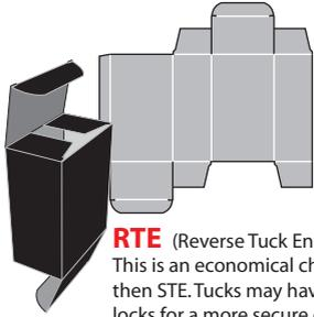
**RTE** (Reverse Tuck End) - This is an economical choice. RTE nests better than STE. Tucks may have either friction fit or slit locks for a more secure closure. Tucks can be on panel two (French Tuck) or panel four (Standard Tuck), depending on presentation preference.
